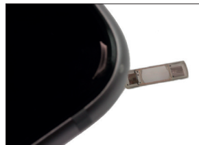
Active eye implant with RF-link
